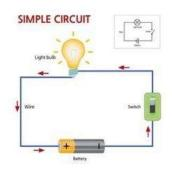
The current flows from negative to positive. There are no gaps - it is a complete circuit and the bulb lights up.
