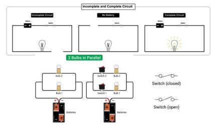
Switches can be placed in a parallel circuit, so that 1 light can be turned on while another is off (just like in a house).
